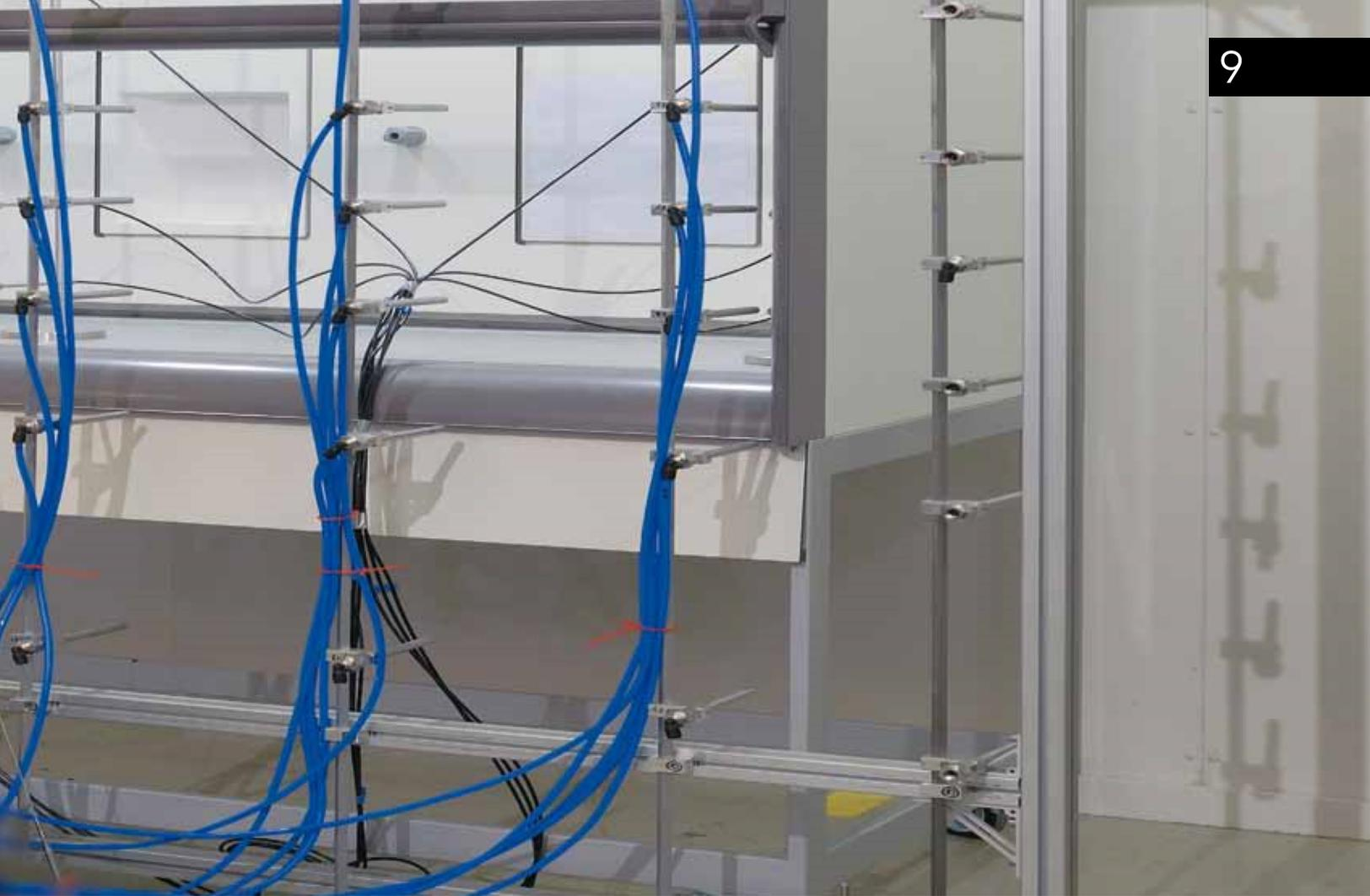
This significantly reduced energy consumption has caused significantly stricter criteria for flow technology in fume hoods. In particular, the new robustness test defines high requirements for the containment values of fume hoods. The robustness test simulates real laboratory conditions by generating frequent movement in front of the hood during the measuring procedure.
