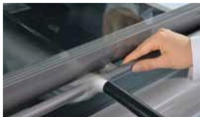
// AIR IS DIRECTED INTO THE FUME HOOD WHEN PUSHING UP THE SASH. THE SASH HANDLE PROFILE IS SHAPED LIKE A SPOILER.
