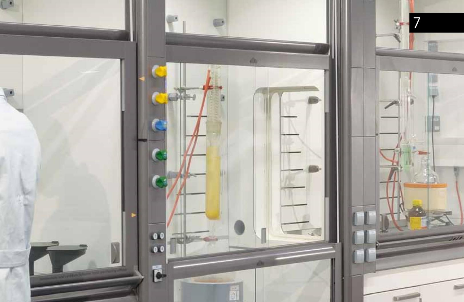
Due to the optimized flow in our new fume hoods, the new Secuflow offers even more safety and requires less energy. When the internal workspace is extensively equipped or a lot of movement is taking place in front of the fume hood, the Secuflow still shows excellent containment values – including when the sash is open. And all this is achieved with reduced exhaust air volumes and, as a consequence, a significantly lower energy consumption.
